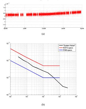
Figure 3. GIOVE System Noise estimation (a): fractional frequency offset over the period Apr 08 – Apr 09, (b): Allan Deviation computed over the last month of data, together with the ground specifications for PHM and RAFS.
