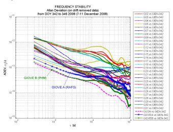
Figure 14. ODTS estimation of Allan Deviation for GIOVE-A (RAFS), GIOVE-B (PHM), and GPS satellites (in pink: System Noise estimation)
