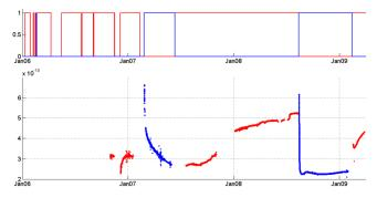
Figure 4. Operation and Performance (Estimated Fractional Frequency Offset) of both RAFS on-board GIOVE-A (red: RAFS-A, blue; RAFS-B).
